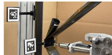
1. Robotic arm locates riveting hole
