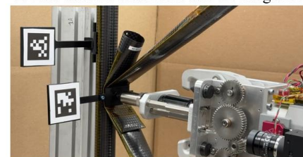
3. Robotic arm guides diagonal to junction and rivet is engaged
