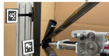
2. End effector is inserted into riveting hole
